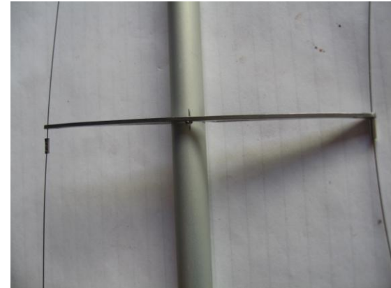
Step 6. Slide crimps onto wires and crimp to keep spreaders level
